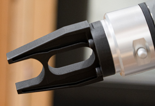
The company has printed end effectors for their robots to conduct numerous tests
